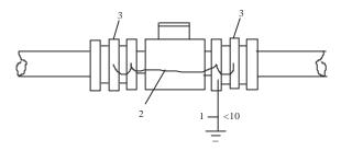
Fig.9.5.1 Installation method on the insulation pipeline
