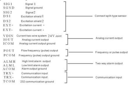
3.3.2 Signal wires processing and labels of connection of square meter and sensor
