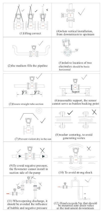
Fig. 9.2 Graphical representation electromagnetic flowmwter installation
