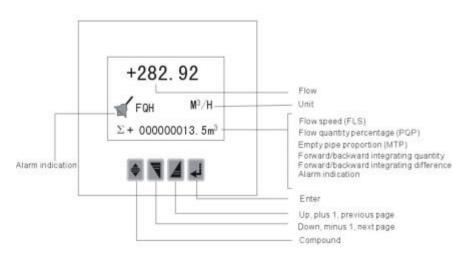
Fig. 3.2.1Keyboard definition and liquid crystal display of square meter 3.2.2 Keyboard definition and liquid crystal display of circular meter
