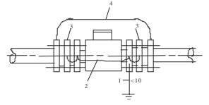
Fig.9.5.2 Installation method of the sensor is on pipeline with cathode protection potential
