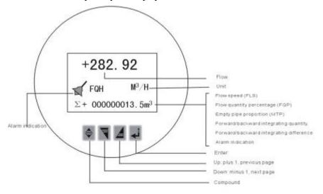
Fig. 3.2.1Keyboard definition and liquid crystal display of circular meter
