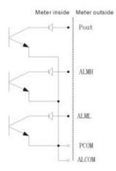
Fig. 3.4 (e) Meter inside OC gate connection mode
