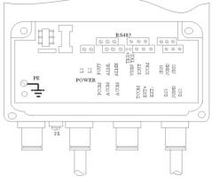
Fig. 3.1 (a) Wiring terminal diagram of square meter
