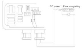
Fig. 3.4 (b) Electromagnetic counter wiring
