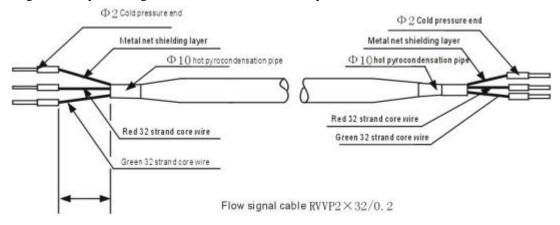
Fig. 3.3.2 Signal wires processing and labels of connection of square meter and sensor 3.3.3 Terminal wiring and labels of circular meter
