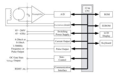
Fig. 2.1 Structure of the converter circuit
